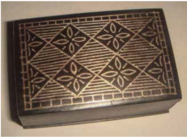
Fig. 17. Small bidri box from the Indian state of Karnataka, inlaid with silver. Bidri consists of 90-92% of Zn and small amounts of Cu and Pb and is patinated in a solution with one part of potassium nitrate, 4 parts of ammonium chloride and one part of sodium chloride. Imported black patinated, inlaid objects of Corinthian type might have suggested the idea for bidri. (Photo by author)
