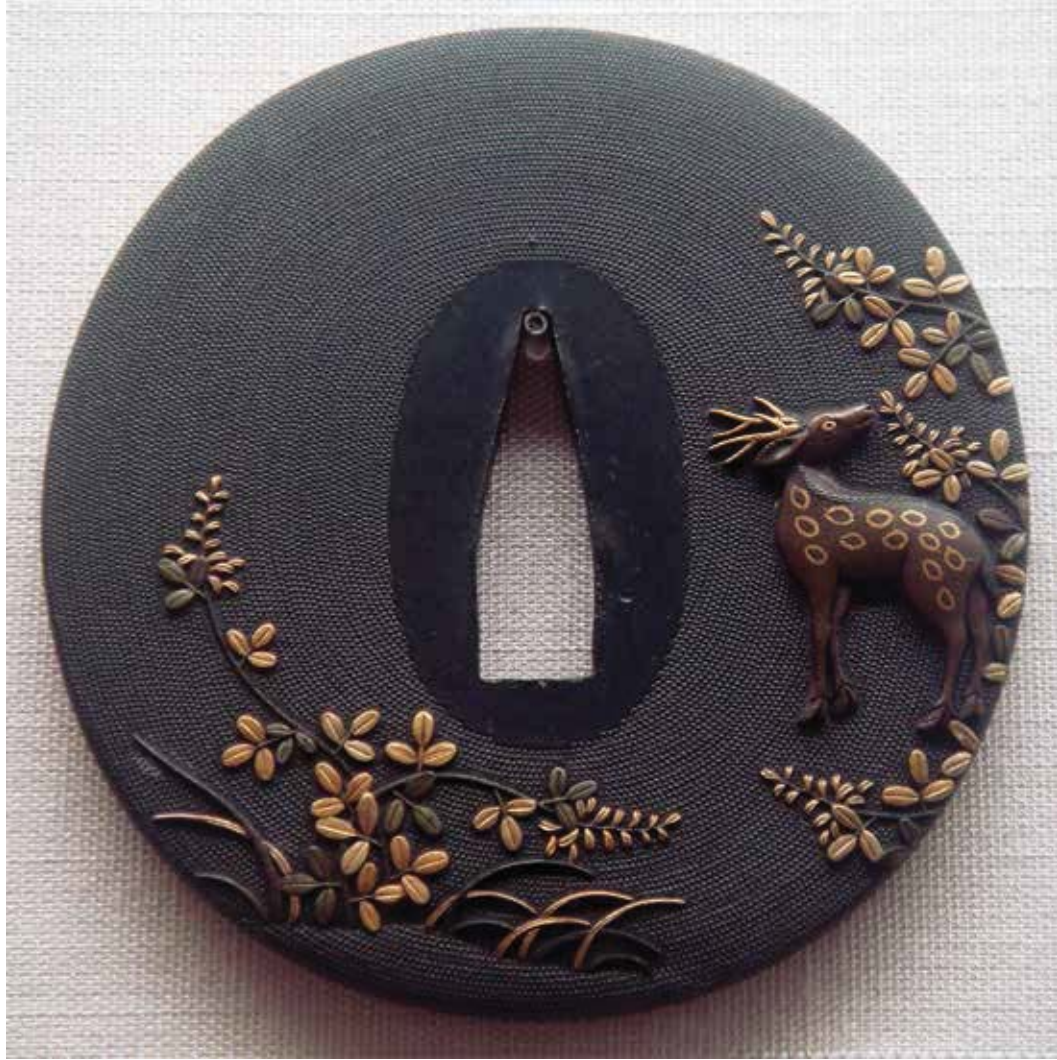
Example of Japanese shakudō, artificially black patinated alloy containing small amounts of gold, treated in a chemical bath to achieve a purple-black or blue-black colour. Tsuba belonging to a daisho (pair of long and short swords) by Kazutomo, Edo period, 19 th century CE. Autumn grass and deer. (Photo by author)
